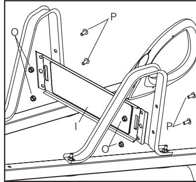
**5** Place leg brace (I) across back of leg and loosely attach using two bolts (P) and nuts (O). Repeat to attach the other end of the leg brace to other leg.
