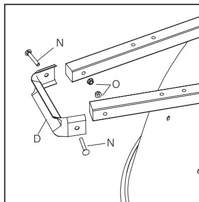
**6** Use two bolts (N) and two nuts (O) to attach wheelguard (D) to front of handles.
