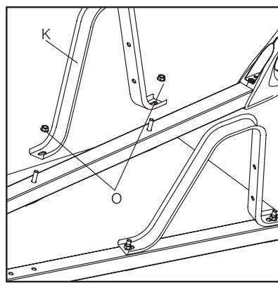
**4** Make sure the holes in leg (K) are facing the back of the tray and then place leg over bolts and loosely attach to handle with nuts (O). Repeat for other leg.
