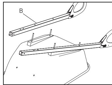
**3** Turn tray over, place handles (B) over bolts and lower onto tray.
