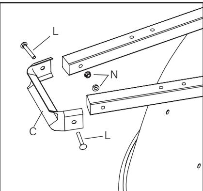
**6** Use two bolts (L) and two nuts (N) to attach wheelguard (C) to front of handles.
