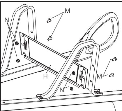
**5** Place leg brace (H) across back of leg and loosely attach using two bolts (M) and nuts (N). Repeat to attach the other end of the leg brace to other leg.
