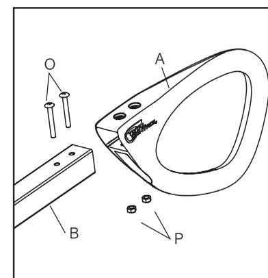
**1** Push Total Control Grip (A) onto end of handle (B) and secure using bolts (O) and lock nuts (P).
