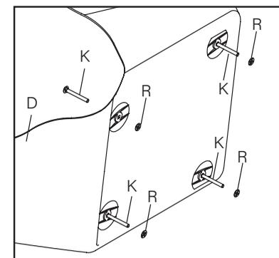
**2** Push bolts (K) through bottom of tray (D) and retainer clips (R).
