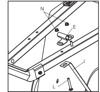
**8** Slide axle (F) through wheel (G) and then into attached bracket. Then slide second axle bracket (E) over other end of axle. Loosely attach second axle bracket and second tray brace to handle. Use bolts (M) and nuts (N) to attach tops of tray braces to tray.
