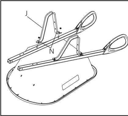
**4** Make sure the holes in leg (J) are facing the back of the tray and then place leg over bolts and loosely attach to handle with nuts (N). Repeat for other leg.
