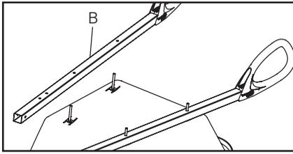
**3** Turn tray over, place handles (B) over bolts and lower onto tray.
