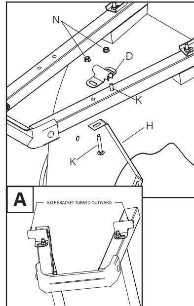
**7** Slide axle (E) through both axle brackets. Slide spacer (O), wheel assembly (F) and washer (P) onto end of axle. Secure by attaching cotter pin (Q) through hole in end of axle. Repeat to attach second wheel. Use bolts (M) and nuts (N) to attach tops of tray braces to tray.
