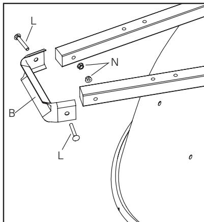
**5** Use two bolts (L) and two nuts (N) to attach wheelguard (B) to front of handles.
