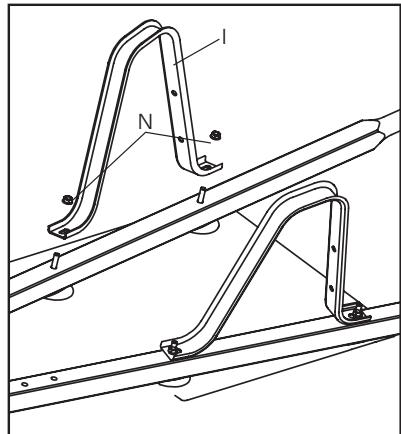
**3** Make sure the holes in leg (I) are facing the back of the tray and then place leg over bolts and loosely attach to handle with nuts (N). Repeat for other leg.
