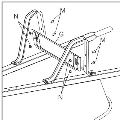
**4** Place leg brace (G) across back of leg and loosely attach using two bolts (M) and nuts (N). Repeat to attach the other end of the leg brace to other leg.
