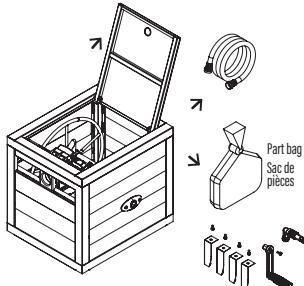
**STEP 2:** Hold the lid closed with one hand, flip the unit upside down and place it on a clean, soft work surface. Install the legs and screws in the bottom corner openings, with the open sides of the legs facing inwards, as shown.
