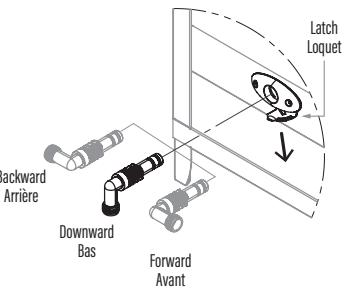
**STEP 5: Make sure the hose guide is lined up with the water system outlet. If necessary, unlock the hose guide by lifting the latch on top of the guide and align it with the water system outlet. Re-lock the hose guide for use.**
