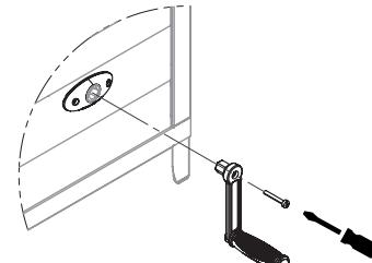
**STEP 4: Install the water system inlet. The water system inlet can face forward, backward or downward. To install, pull the latch downwards, insert the water system inlet in the desired direction and lock it in place by pushing the latch back into its original position.**
