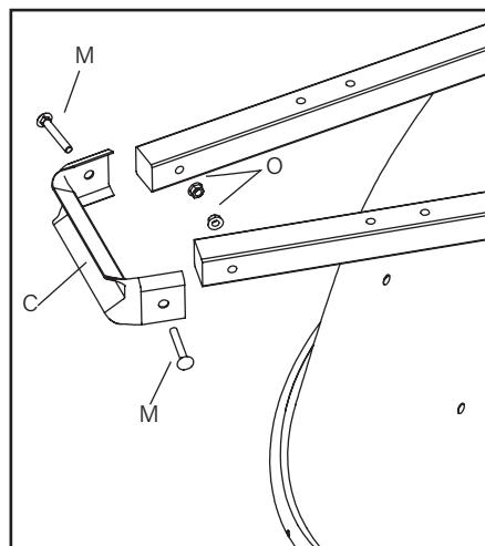
**5** Use two bolts (M) and two nuts (O) to attach wheel guard (C) to front of handles.
