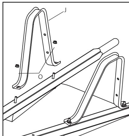
**3** Make sure the holes in leg (J) are facing the back of the tray and then place leg over bolts and loosely attach to handle with nuts (O). Repeat for other leg.
