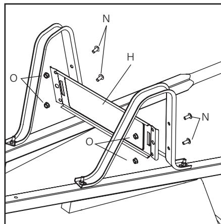
**4** Place leg brace (H) across back of leg and loosely attach using two bolts (N) and nuts (O). Repeat to attach the other end of the leg brace to other leg.
