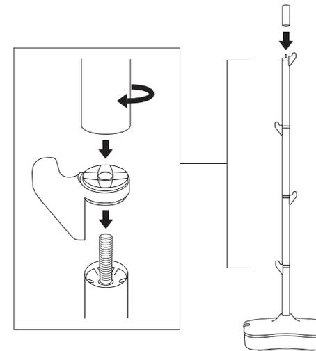
Continue with a second long tube (4), and repeat the previous step for each of the three remaining hooks. Finish by screwing the short tube on top of the pole (5).
