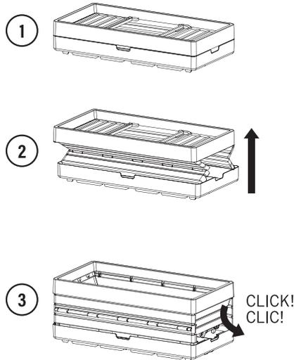
Make sure the front panels are completely unfolded and the side ones well clipped to the base.
