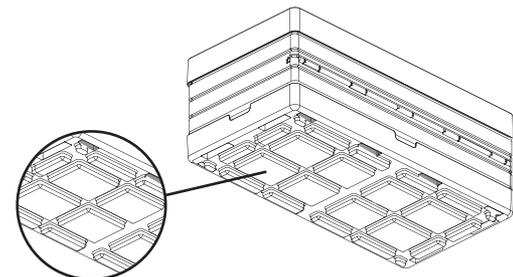
You can adjust the width of your modular structure by simply selecting the appropriate slot.
